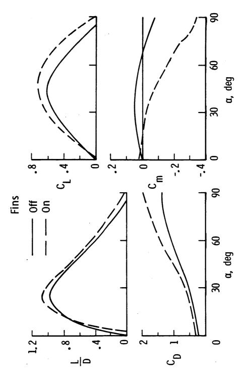
Figure 20.- Longitudinal characteristics, lenticular body, M = 2, c. g. = 0.45  $\alpha$ .
