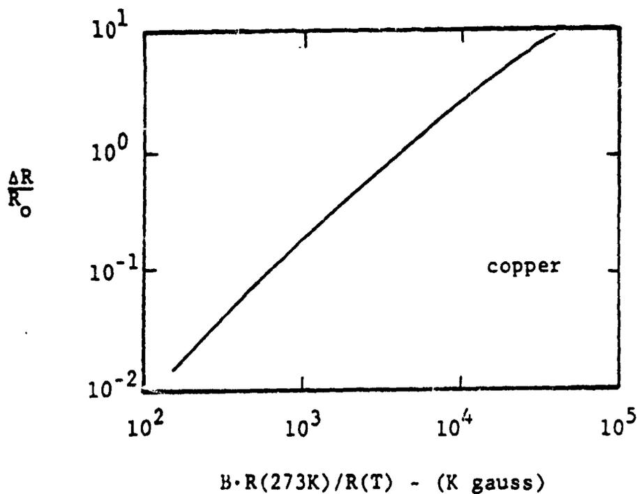
Thus, it would appear that the dominating factor in the increase of resistivity due to the magnetic field would be the purity (RRR) of the copper. A practical value of resistivity at 27K would probably lie somewhere between the two examples above and thus the problem of an increase in resistivity due to a magnetic field and hence a decrease in the damping coefficient should not be a severe or overriding concern.
