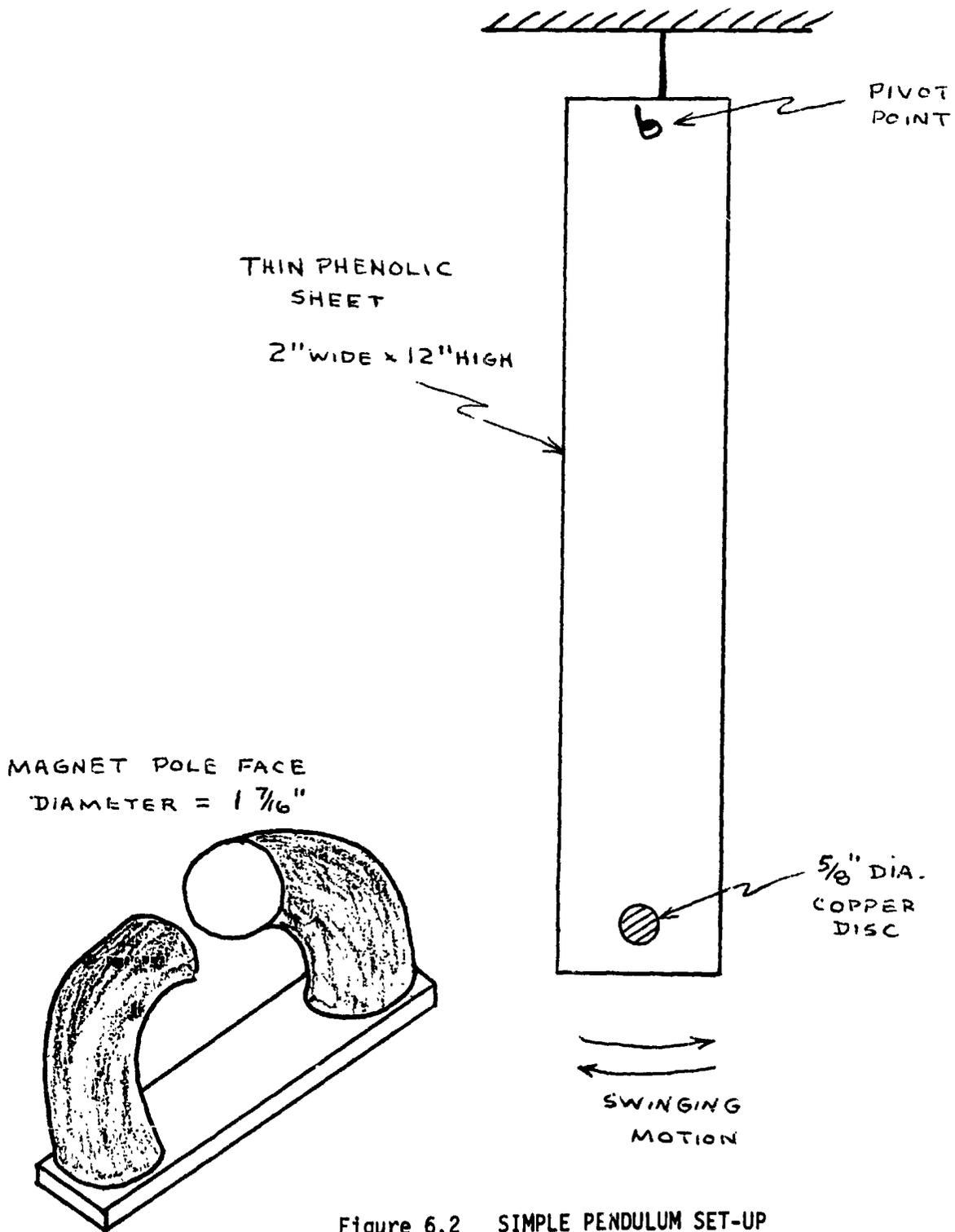
Figure 6.2 SIMPLE PENDULUM SET-UP
