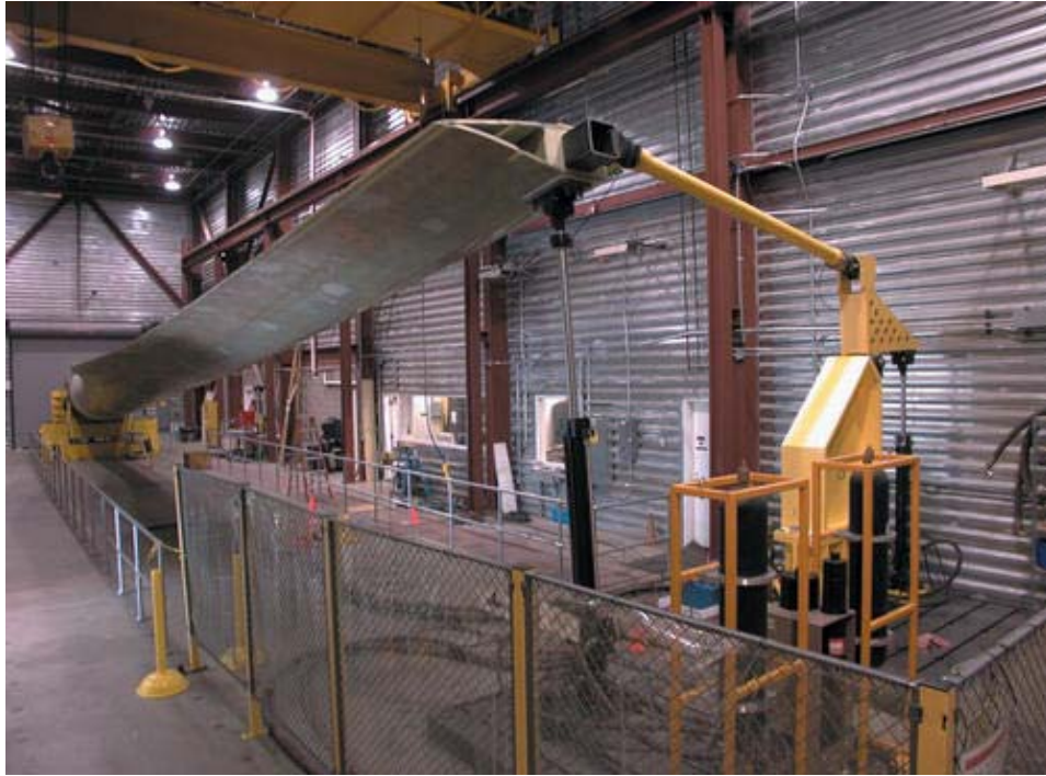
Figure 1. NREL's dual-axis force-displacement fatigue test
