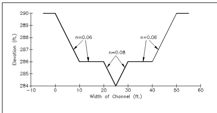
Figure 5.1. Example cross section.
