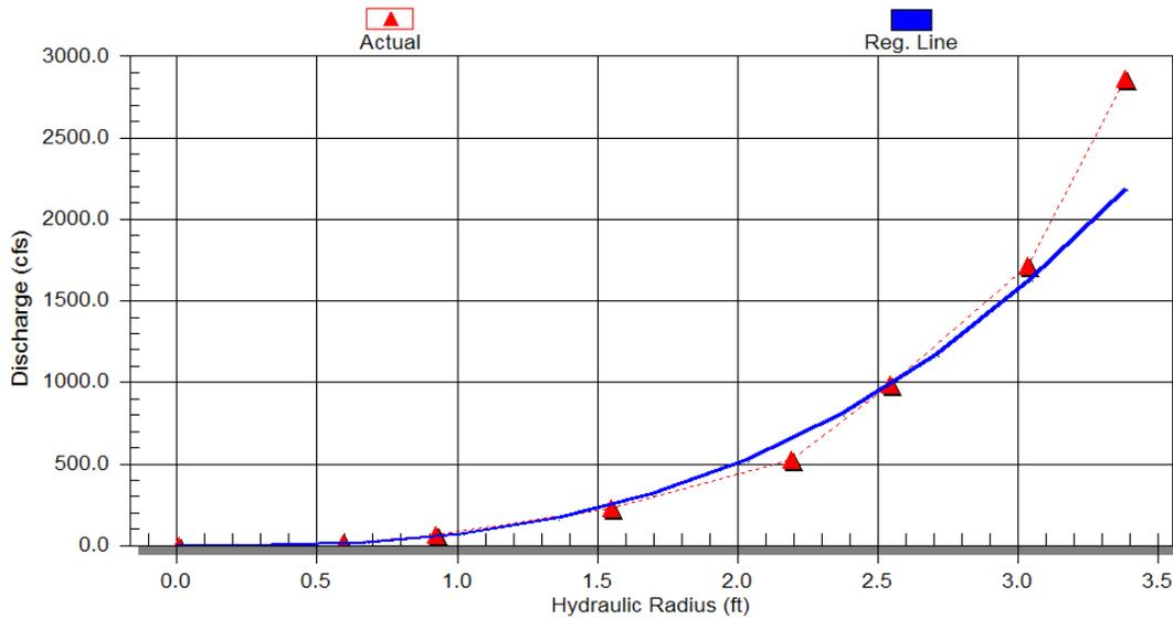
Figure 5.13. Discharge vs. Hydraulic Radius Regression Curve.
