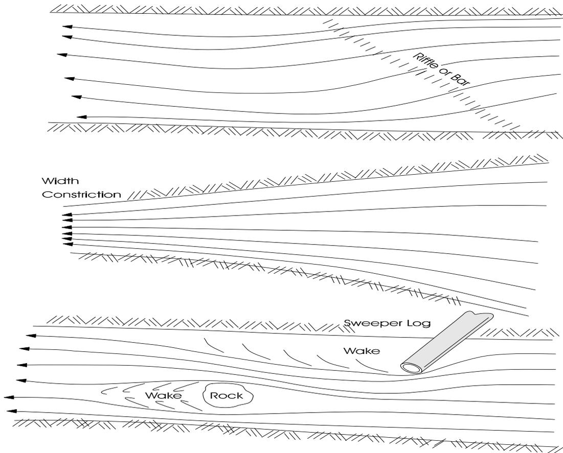
Figure 2.2. Typical channel configurations that disrupt uniform flow.
