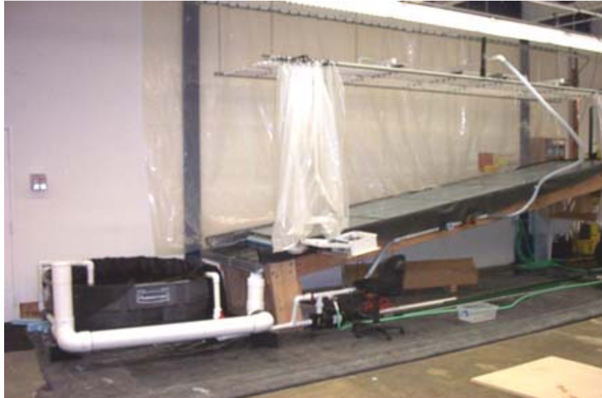
Figure 15: Drainage Test Setup
