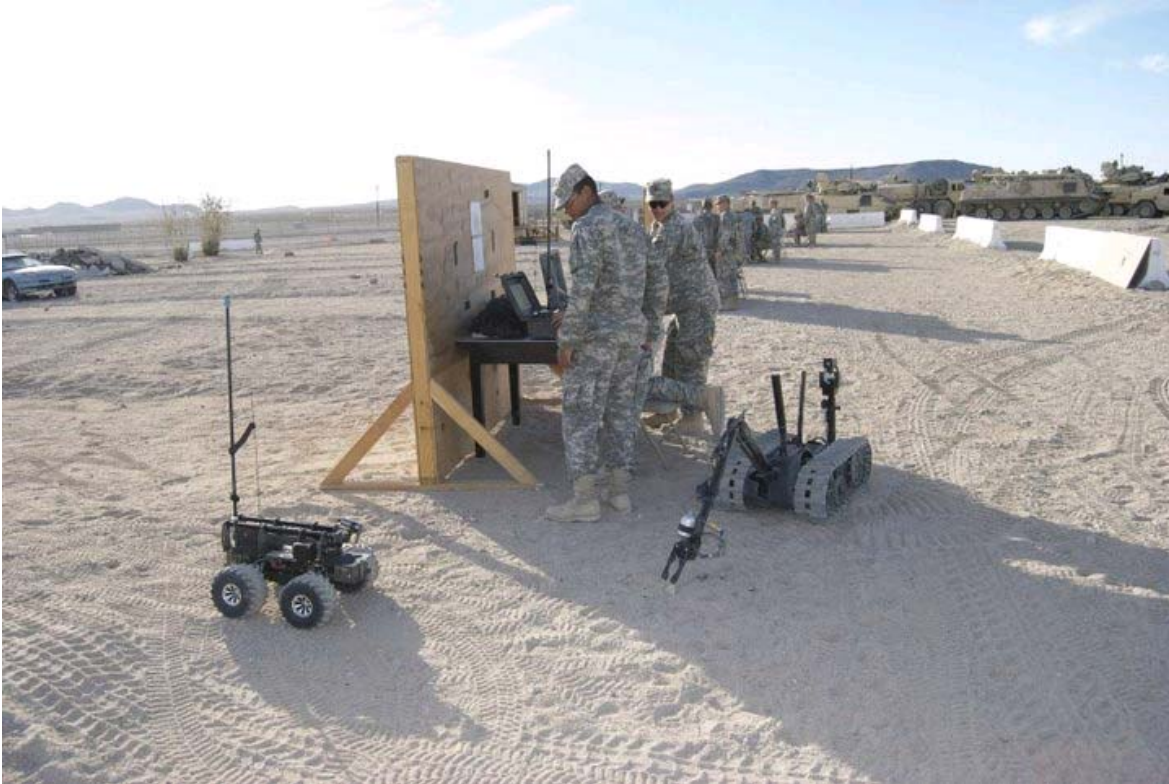
Robotics training at the National Training Center at Fort Irwin, California. The robots used here are the MARCbots. Talons and PackBots are also used in the C-IED fight.
