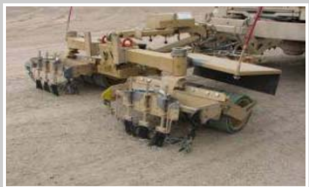
Another JIEDDO initiative is the Wire Neutralization System-Wolf Collar for raking up command wires used to trigger IEDs. JIEDDO has spent $67 million on this initiative.
