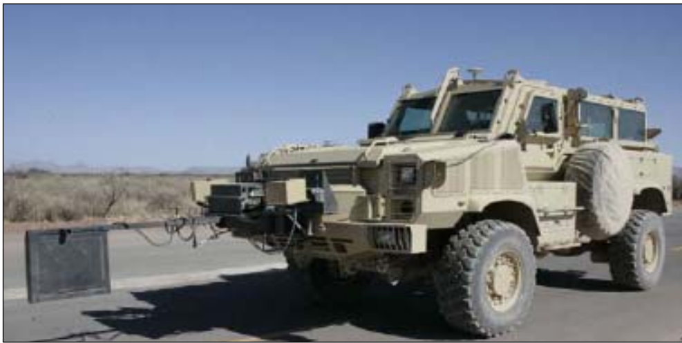
One initiative JIEDDO has transferred to the Services is the "Rhino," a vehicle-mounted system to pre-detonate IEDs.
