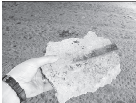
Concrete that Fell from Flume
