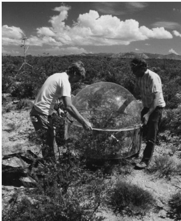
Figure 1. Chamber operation in sparse canopy. Chamber being lowered over creosote bush. Eddy correlation sensors in left background.
