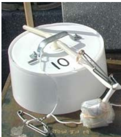
Figure 3. Seepage meter (~10.5 inches diameter) with clip for transect line and folded bag
