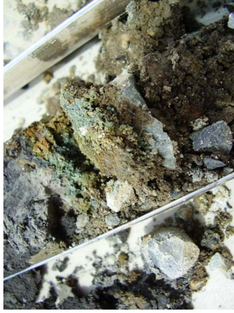
6/5/06 Closeup of Maintenance Area sample MAINT-1-16. Note green discoloration of soil.
