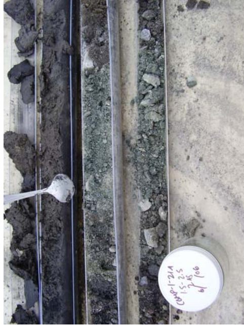
6/8/06 Closeup of Compressor Area sample COMP-1-21. Note green soil horizon.
