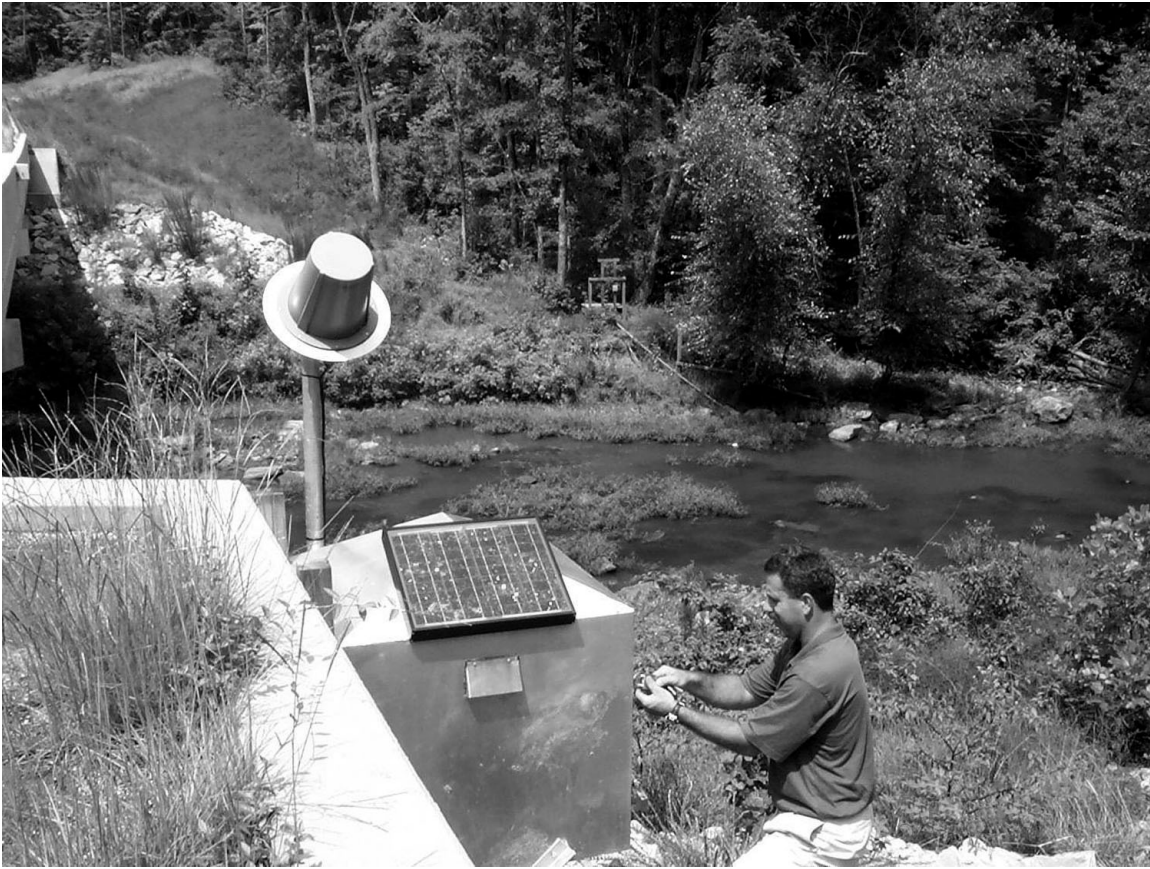
Gaging station at Little River at state road 1461 near Orange Factory, North Carolina.
