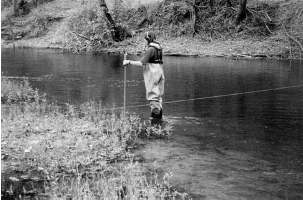
USGS hydrographer making a wading discharge measurement at Neuse River near Falls.
