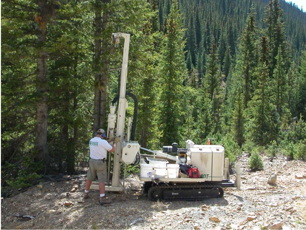
Figure 9. Geoprobe model 5410D rig near the mouth of Prospect Gulch (GPPG-10) operated by the U.S. Geological Survey under Bureau of Land Management contract.
