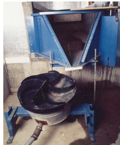
H Flume and Coshocton Wheel for Measuring and Sampling Surface Water Runoff
