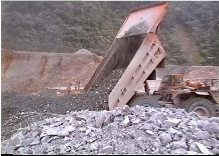
Figure 2. Truck depositing mine waste from an open pit copper mine in Papua New Guinea (Forderkreis >> Rettet die Elbe << eV, 2001).
