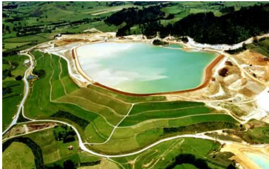
Figure 5. Tailings storage facility at the Martha Mine near Waihi, New Zealand, nearing its final height. This aerial photograph,
