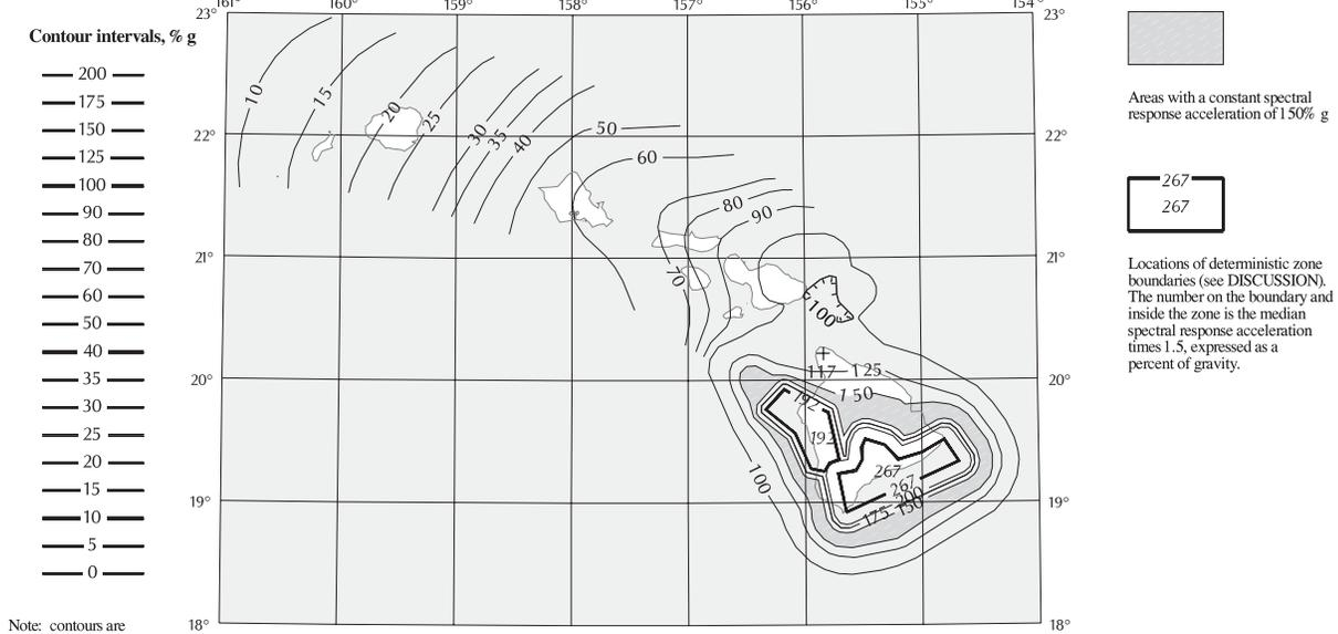
**0.2 SEC SPECTRAL RESPONSE ACCELERATION (5% OF CRITICAL DAMPING)**
