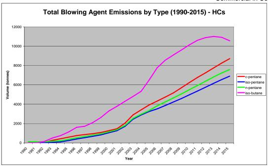
It is interesting to note that iso-butane has greater emissions than the other hydrocarbons even though its usage is less. This reflects its use in emissive applications such as polyethylene slab applications where short-term emission is required for safety reasons.
