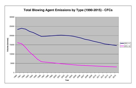
The slow release of blowing agent from the banked blowing agents in construction foams is combined with the peaks of emissions from the tail of CFC consumption in 1990/91 and domestic refrigerators decommissioning (2002/03) in the above graph
