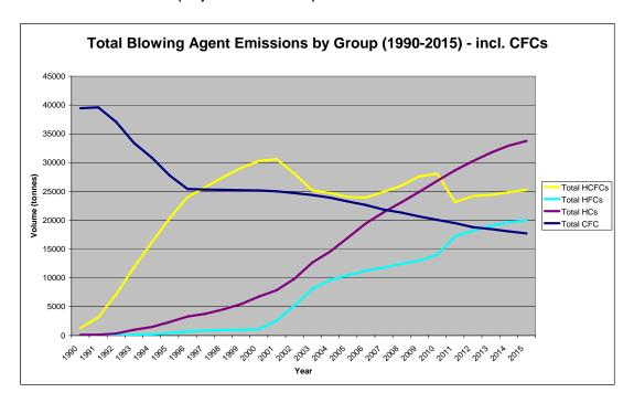
The importance of emission functions, however, should not be under-estimated when considering the emissions of blowing agents used in only a few sub-sectors. Accordingly, the emission assumptions for XPS have a significant bearing on HFC forecasts. In order to ensure a pessimistic view of HFC emissions, the emission function adopted for XPS have been higher than the industry is currently predicting.
