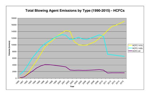
The significant increase in HCFC-141b emissions in the period from 2005 is caused mostly by the decommissioning of North American domestic appliances. The drop in HCFC-142b emissions in 2010 coincides with the phase-out on consumption in the XPS Board sector – a fairly emissive manufacturing process.
