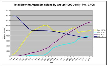
The on-going impact of CFC emissions from banked blowing agent is clearly evident from the graph. Although this falls below the emissions for HCFCs and latterly HFCs, it should be noted that very little end-of-life decommissioning is considered for building applications during the period of this study (1990-2015). Accordingly, there is expected to be a further growth in emissions arising from CFCs after 2015 as products installed from 1965 onwards begin to be decommissioned.
