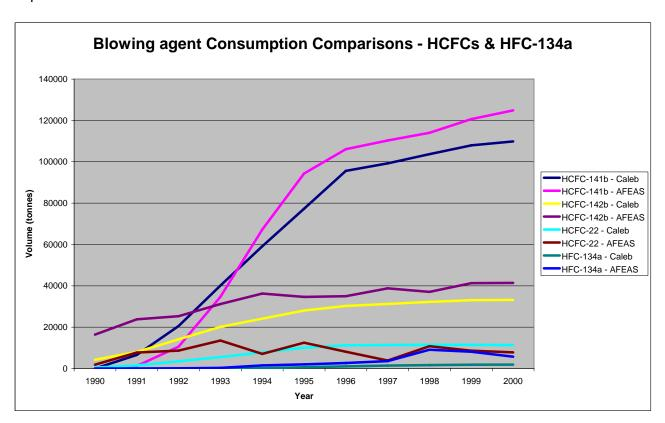
For HCFC-141b, the comparison to 1993 shows the conversion from CFC-11 to be slightly more progressed than it actually seems to have been from AFEAS data. However, based on a peak CFC-11 consumption of 140,000 tonnes, errors of less than 10,000 tonnes in periods of high transition activity should be broadly acceptable in a model of this type.
