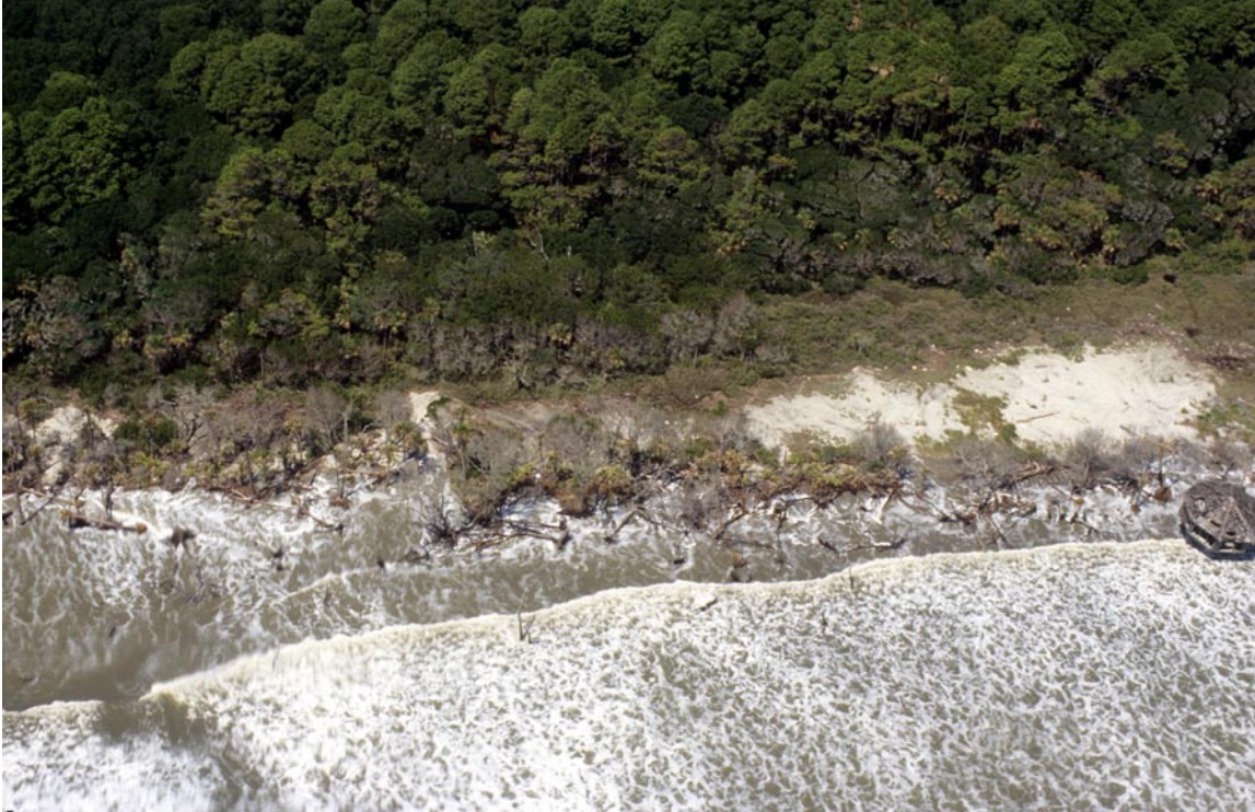
Figure 17. Dead and fallen trees and beach houses in the surf zone are indicators of long-term beach erosion. This example is from Pritchards Island, South Carolina.
