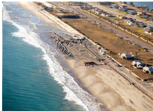
Figure 19. Many beaches along the east coast of Florida, such as this one at Patrick Air Force Base, have been nourished to mitigate against long-term erosion. Photo provided by the Minerals Management Service.
