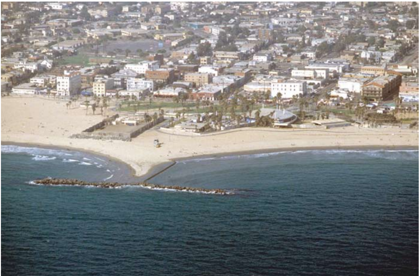
Figure 38. Oblique aerial photograph of a breakwater along the highly engineered Santa Monica coastline (Copyright © 2002-2005 Kenneth & Gabrielle Adelman, California Coastal Records Project, www.californiacoastline.org ).
