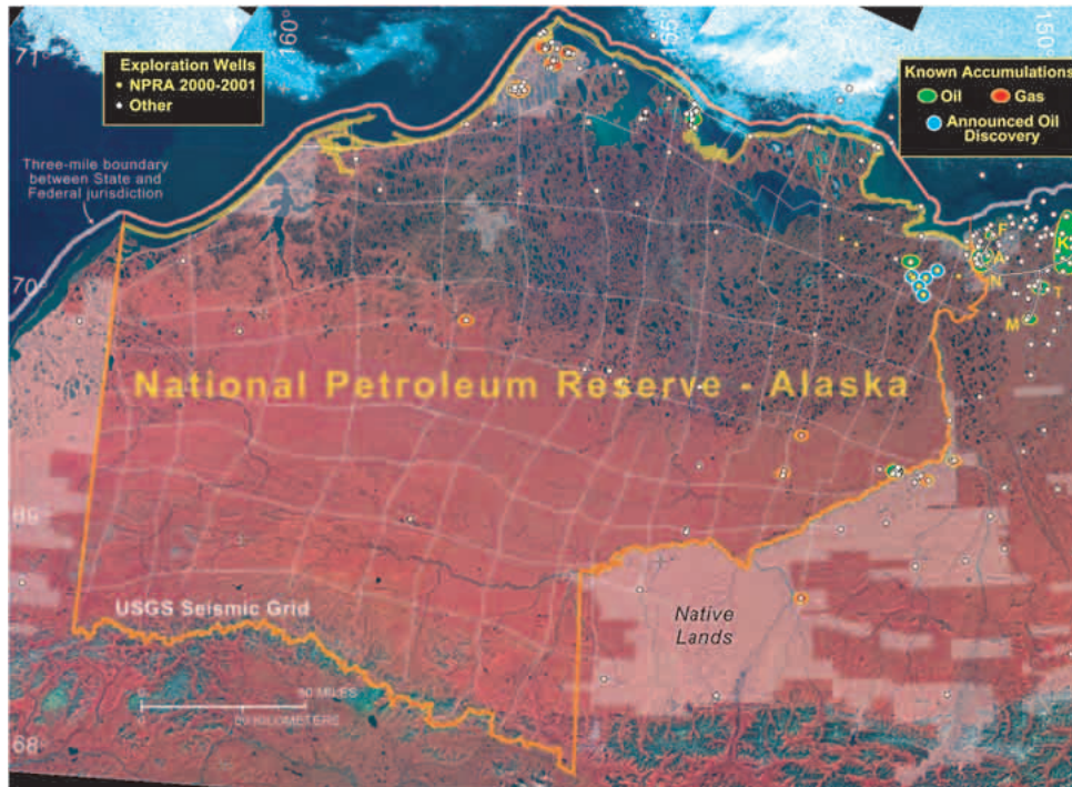
Figure 2. Map of the National Petroleum Reserve in Alaska (NPRA; boundary shown by yellow line) and surrounding region with locations of seismic lines, wells, oil and gas accumulations, and Native lands. Red line shows the total area assessed in 2002 by the U.S. Geological Survey (USGS), including Federal and Native lands and State offshore areas. USGS seismic grid shows location of those seismic lines reprocessed and reinterpreted for this assessment. The assessment incorporated information on all exploration wells except those in the northeast part of NPRA drilled during 2000 and 2001. Oil fields east of NPRA, including several recently discovered accumulations, are labeled as follows: A, Alpine; F, Fiord; K, Kuparuk River; M, Meltwater; N, Nanuq; and T, Tarn. The map base is a false-color composite Landsat image on which vegetation appears as shades of red, and soil and rock with little or no vegetation appear in shades of green and brown. Deep and clear water appears dark blue to black, and shallow or sediment-laden water appears in lighter shades of blue. Ice is white or bluish white.
