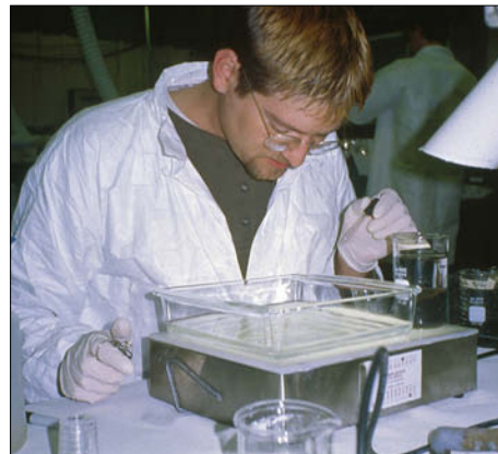
Sediment toxicity test development requires establishing standard procedures such as seen above, placing test organisms into test beakers.
