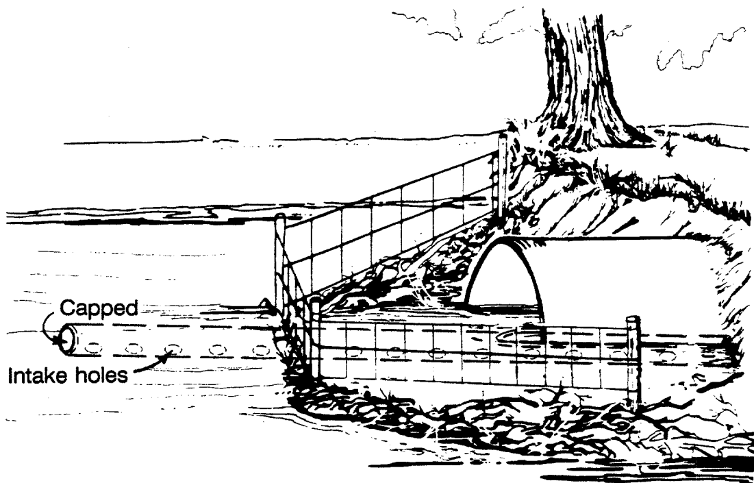
Figure B.24.1. The perforated pipe method.
