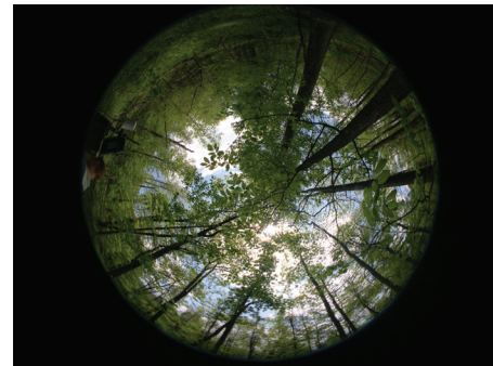
Figure 3. Periodic photographs taken from beneath the canopy using a skyward-facing fish-eye lens can be used to measure when leaves come out and how much tree cover exists at specific locations.
