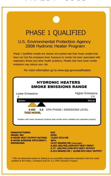
The U.S. Environmental Protection Agency (EPA) has updated its voluntary program to rate hydronic heaters. Models with the white tag meet EPA's Phase 2 emissions level. These heaters meet stricter guidelines and pollute less. Heaters with the white tag have been tested by an EPA-accredited laboratory and are 90% cleaner than unqualified models. (Orange tag models are 70% cleaner than unqualified models.)
