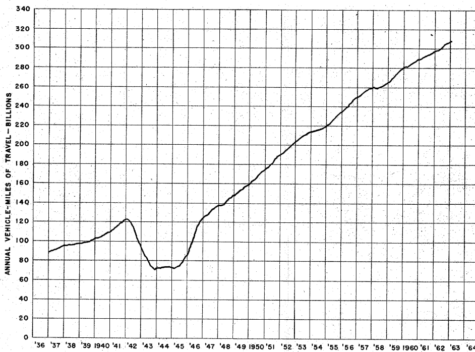
FIGURE 2-- TRAVEL ON MAIN RURAL ROADS BY 12-MONTH PERIODS ENDING EACH MONTH, IN VEHICLE-MILES
