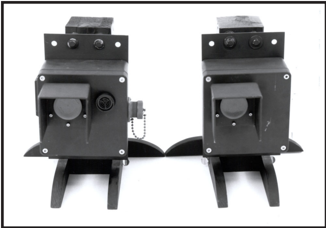
Figure 3—Ivan Technologies trail traffic counter.
