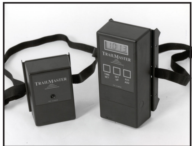
Figure 4—TrailMaster TM1000 trail monitor system.
