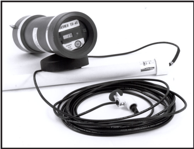
Figure 9—The PR-40 sensor has a geophone attached to a plastic PVC pipe rather than a mat.
