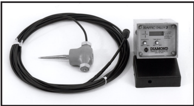
Figure 10—Diamond Traffic Products' TT-3 traffic counter.
