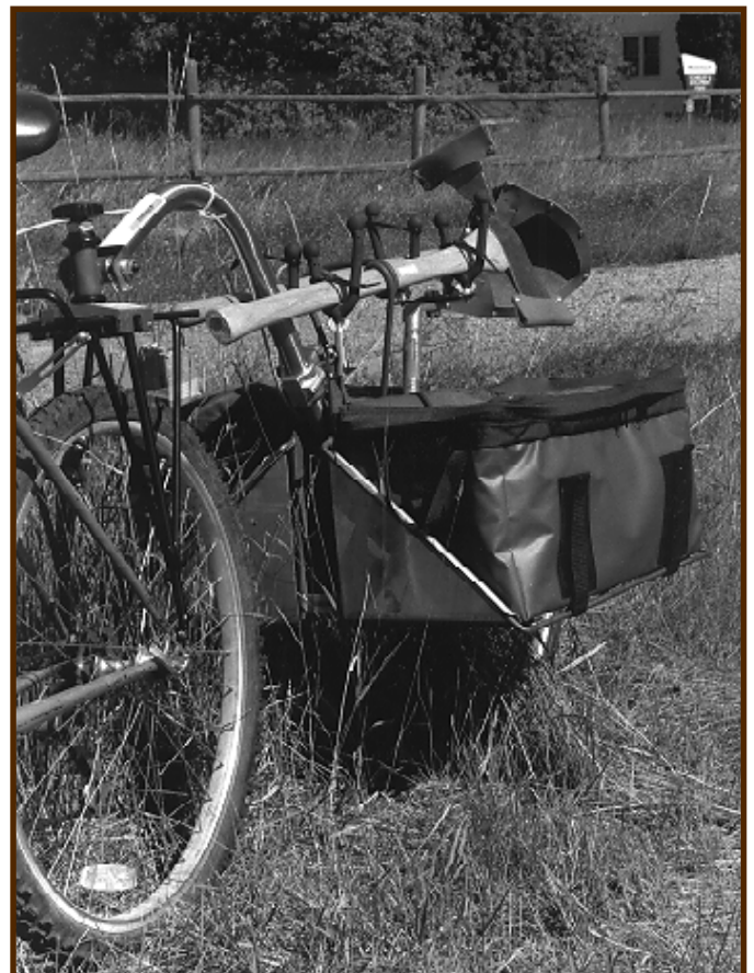
Figure 13—We used steel and accessories designed for ATV's, but neglected to consider the importance of using lightweight materials.
