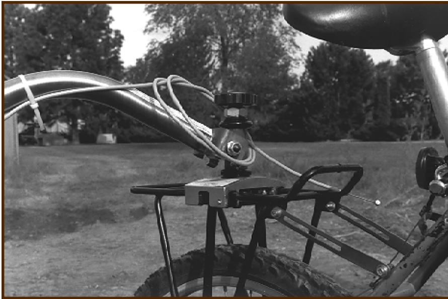
Figure 11—Burley's hitch and pivot system and Moose Rack are used in their Piccolo trailercycle. The cables are for a brake on the MTDC prototype trailer.
