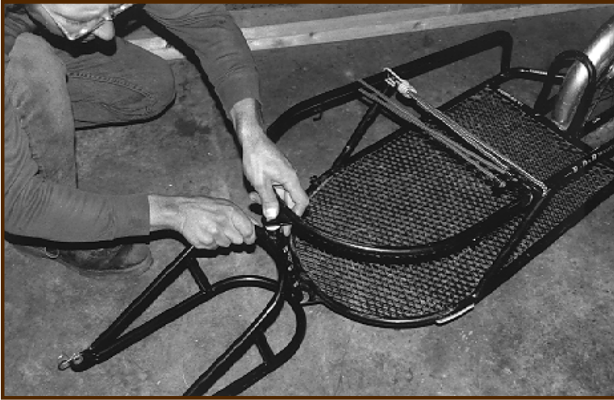
Figure 7—The pivot rod (under his thumb) bent on this B.O.B. Yak. On new models, the manufacturer is using a larger diameter rod and the pivot rod nut is sealed with Loctite to keep it from loosening.
