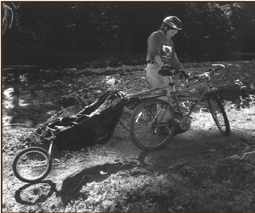
Figure 10—The Wheelee Pac Dog is long and tracks wide around curves, a disadvantage.
