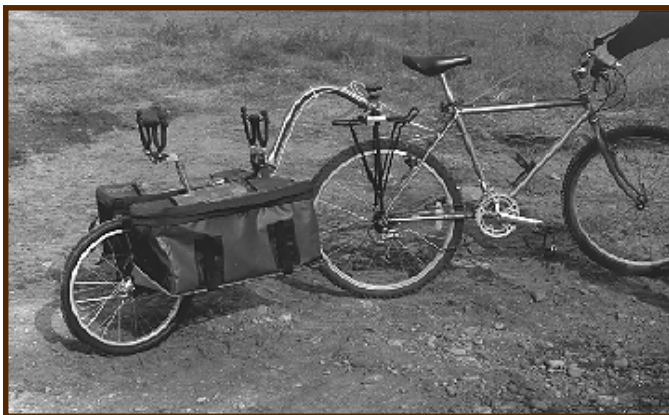
Figure 12—Clueless in Missoula. We put too much emphasis on sturdiness and not enough on reducing weight. You'll need a locomotive to pull this 40-pound beast.
