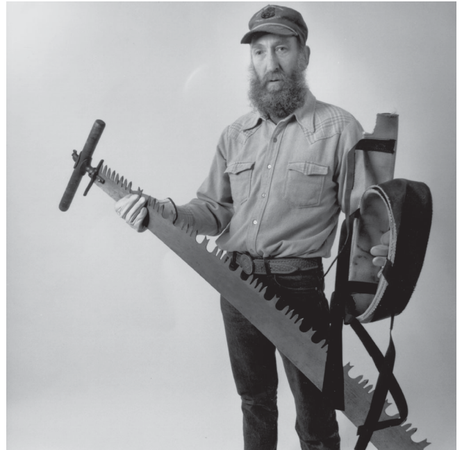
Figure 7—The sawguard is rolled and ready to be applied to the saw.
