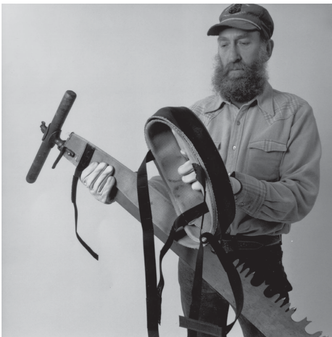
Figure 8—Unrolling the sawguard along the saw's cutters.
