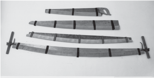
Figure 2—Crosscut saw guards properly applied using 1-1/2-inch fire hose. Velcro-style fasteners secure the straps.
