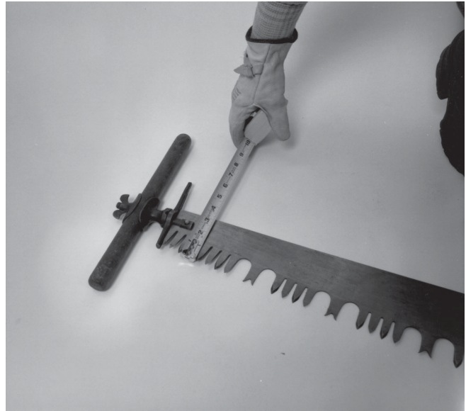
Figure 4—Measuring the width of the saw from the cutters to the back.
