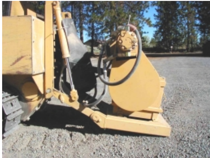
Figure 5—Notice the mud flap attached to the back of the Sweco.
