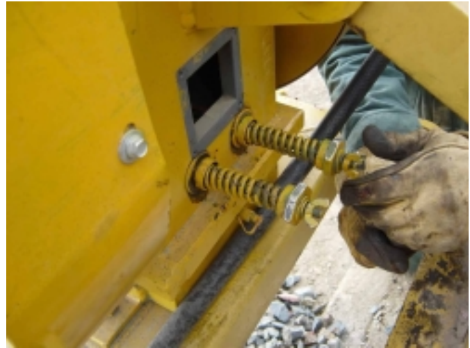
Figure 3—Tightening tensioner rods after adjustment of jaw.
