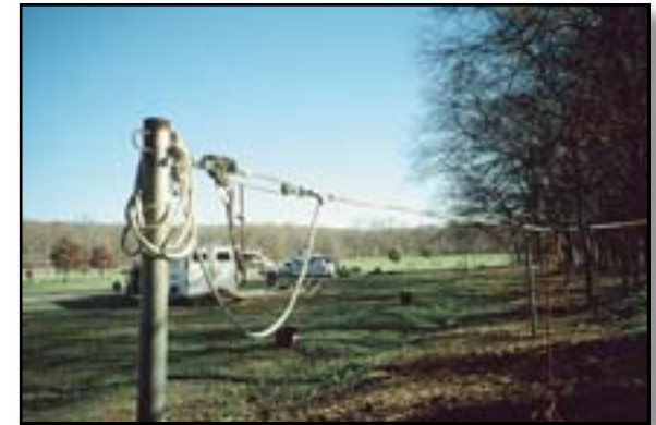
Figure 10–54—To be effective, highlines must be stretched taut. A hand winch helps to apply enough tension.
