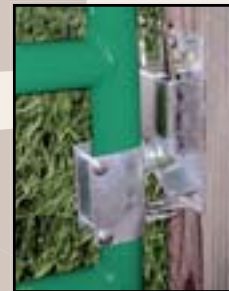
Figure 10-35— This latch allows the gate to swing both ways, can be opened from horseback, and supports the closed gate. — Courtesy of Co-Line Welding, Inc.
