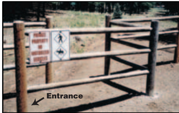
Figure 10-30—Chicanes use tight turns to prevent unauthorized use. The entrance to this modified chicane is immediately left of the signs.
