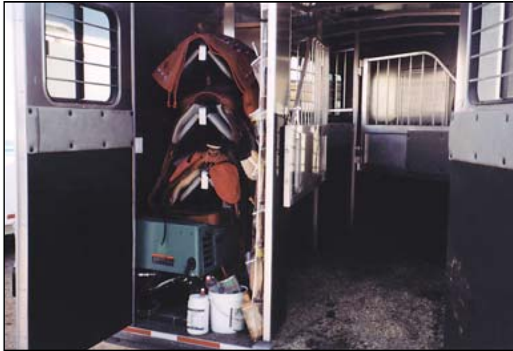
Figure 9-7—Horse trailers, such as this slant-load model, often have tack storage that is accessed through side or rear doors.
