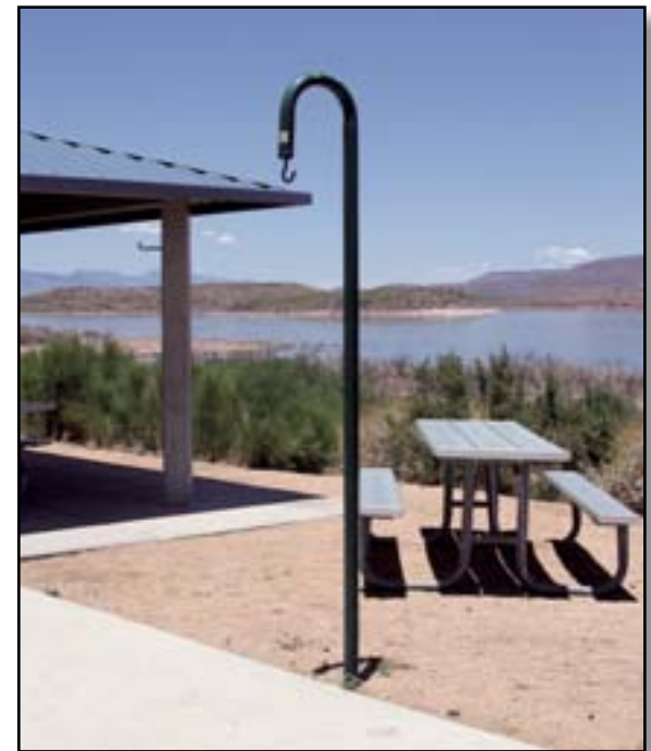
Figure 9–23—For lantern hangers to be accessible, they should not be more than 48 inches from the ground. This style of lantern hanger could be adapted by adding a second, lower hook.
