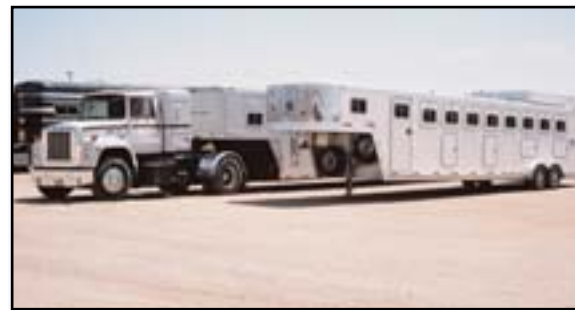
Figure 8–11—Some vehicles carry up to eight horses, contain living quarters, and include storage space.
