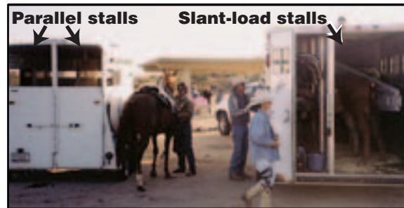
Figure 8-7—Saddling a horse or mule requires access to all sides of the animal, and tight quarters make the job difficult. Note the difference in the horse trailers. The trailer on the left has parallel horse stalls, and the trailer on the right has slant-load —or angled—stalls with a storage area behind the partially closed door.
