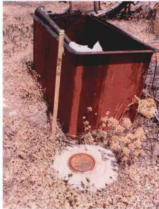
Monitoring well W-16
