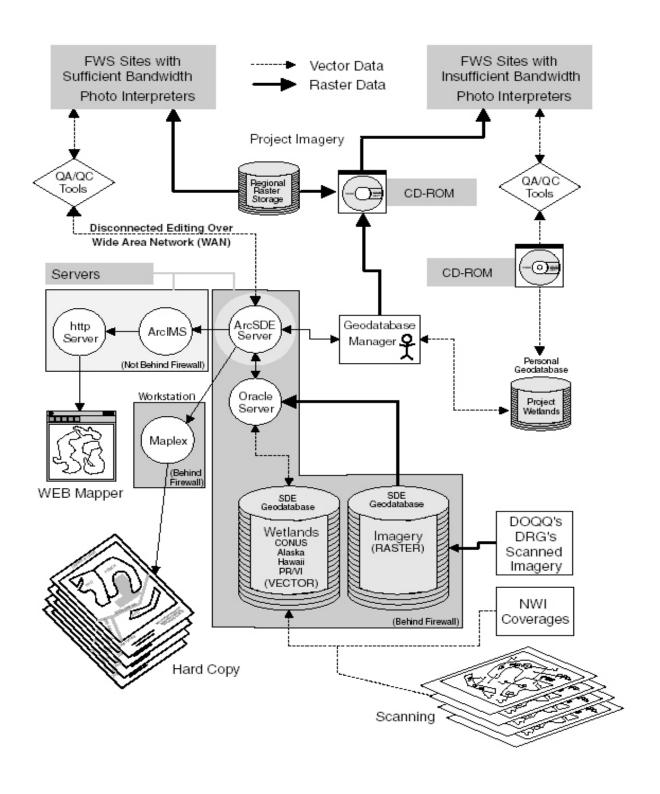
Figure 4. Data flow diagram for the Wetlands Master Geodatabase (This illustration has been simplified for display purposes).
