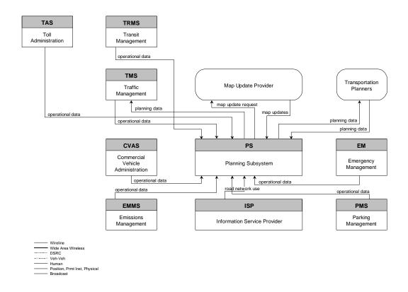
Figure 1.2. Architecture Flow Diagram for the Planning Subsystem
