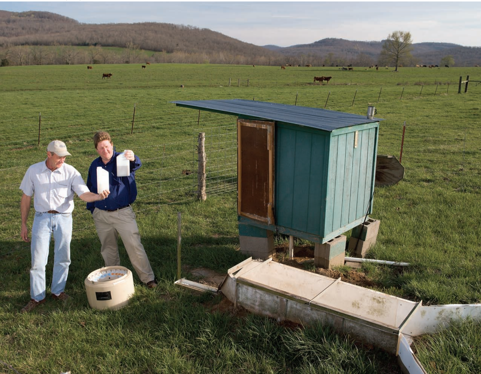
Technician Scott Becton (left) and soil scientist Philip Moore collect runoff water samples from a long-term paired watershed study being conducted in northwest Arkansas to measure phosphorus runoff from alum-treated poultry litter.
