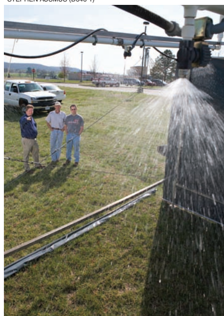
ARS and University of Arkansas scientists conduct a rainfall simulation to determine the long-term effect of alum-treated poultry litter on aluminum and phosphorus runoff.
