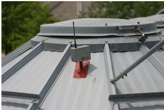
Radio transmitter receiving signals from sensors in grain bin.
