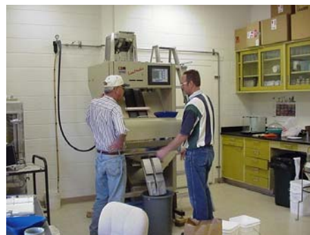
High speed sorting system for purifying large samples for breeding programs.
