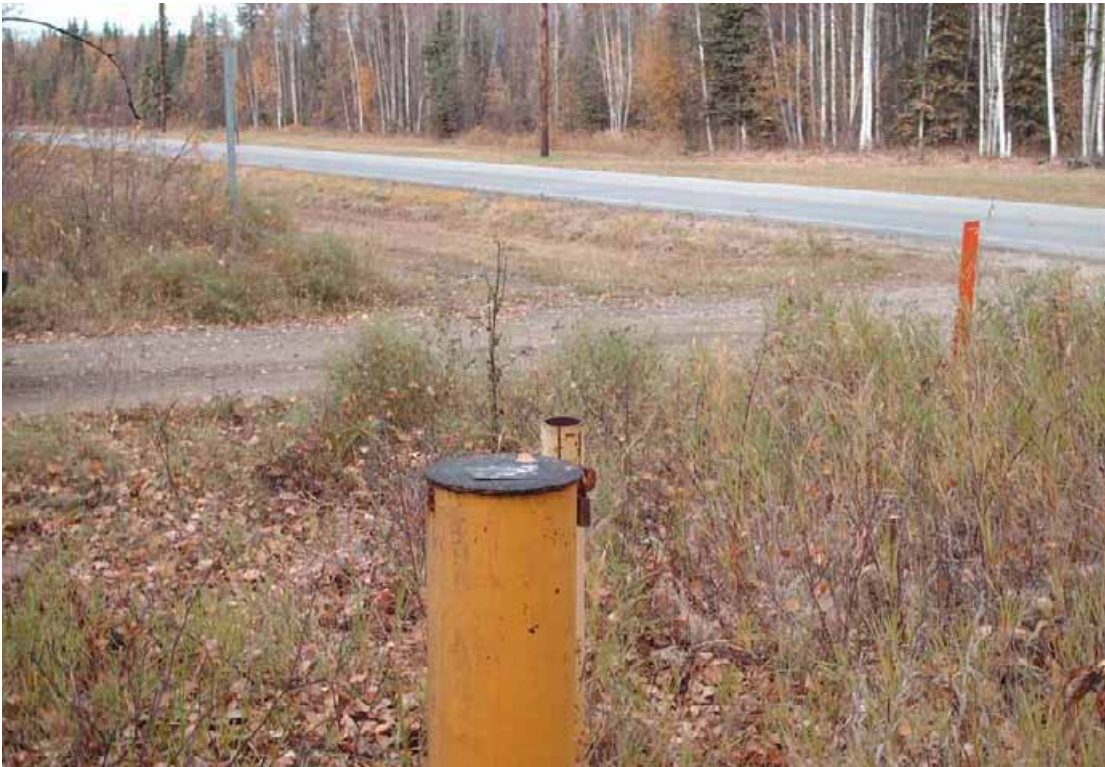
Photograph 22 – Monitoring Well AP-6132 (Upgradient from Landfill) Operable Unit 4
