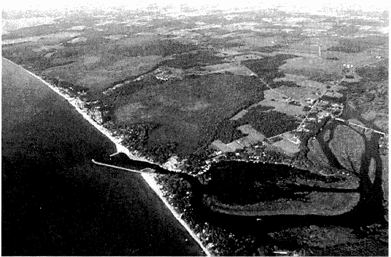
Plate 4c. Barred estuary at Salmon River, NY. Longshore transport has nearly barred this estuary by depositing a barrier dune across its mouth, slowing river discharge into Lake Ontario and forcing the river to meander broadly. The opening at the river mouth is now maintained by jetties. (Photo by John Griebisch 1990).
