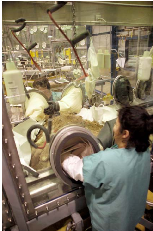
Figure 10-16. Glovebox excavator operators segregating waste retrieved from Pit 9.
