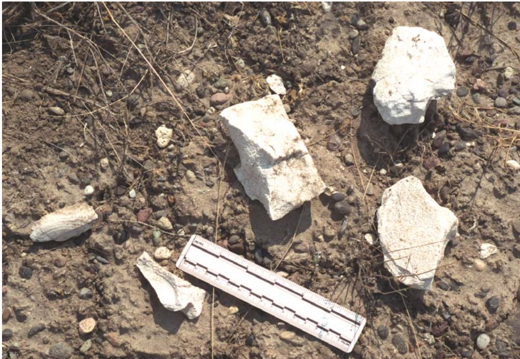
Figure 18. The top photograph shows a large metal fragment remaining from a bomb and chunks of TNT. The bottom photograph shows chunks of RDX.
