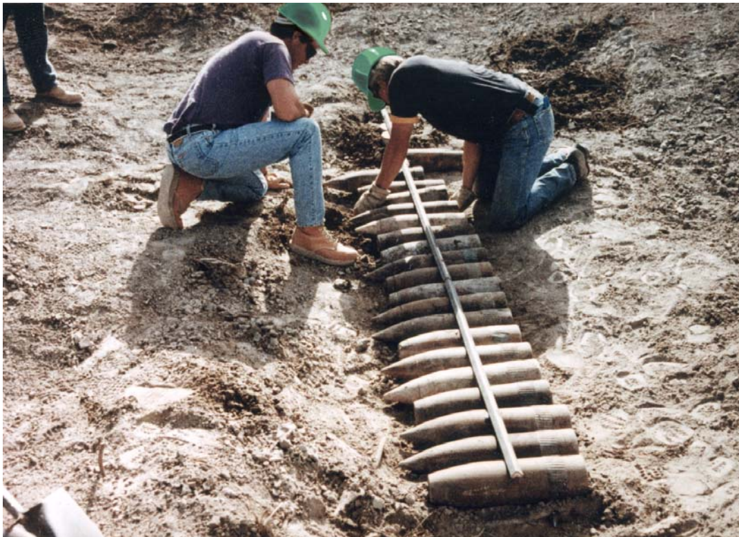
Figure 14. The top photograph shows a stack of five projectiles found along Power Line Road. They consist of two 5-in. and three 2-in. projectiles assumed to be non-explosive. Evidence of firing is shown near the end of the projectile by the rifling pattern in the rotating band. The bottom photograph shows a collection of projectiles being prepared for demolition using a flex-linear shaped charge at the MDA.
