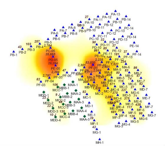
The following site map illustrates the locations of the passive soil gas samplers (yellow triangles) installed in the western side of the site in June 2008. Tetrachloroethene was only detected in one sampler.
