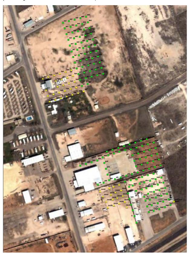
The following site map illustrates the detections of tetrachloroethene in the passive soil gas samplers installed at the south side of the site (see site map above). The blue triangles and green diamonds mark the location of individual samplers (see site map above). The passive soil gas samplers installed on the north side of the site did not detect tetrachloroethene or any of the other contaminants of interest at the site.
