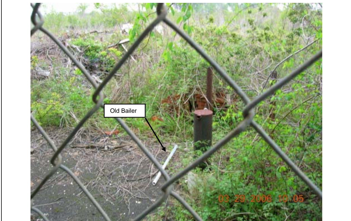
Photo 4: View of monitor well MW-11, located on north side of Process Building No. 2. An old bailer, used for sampling, is lying next to the well.
