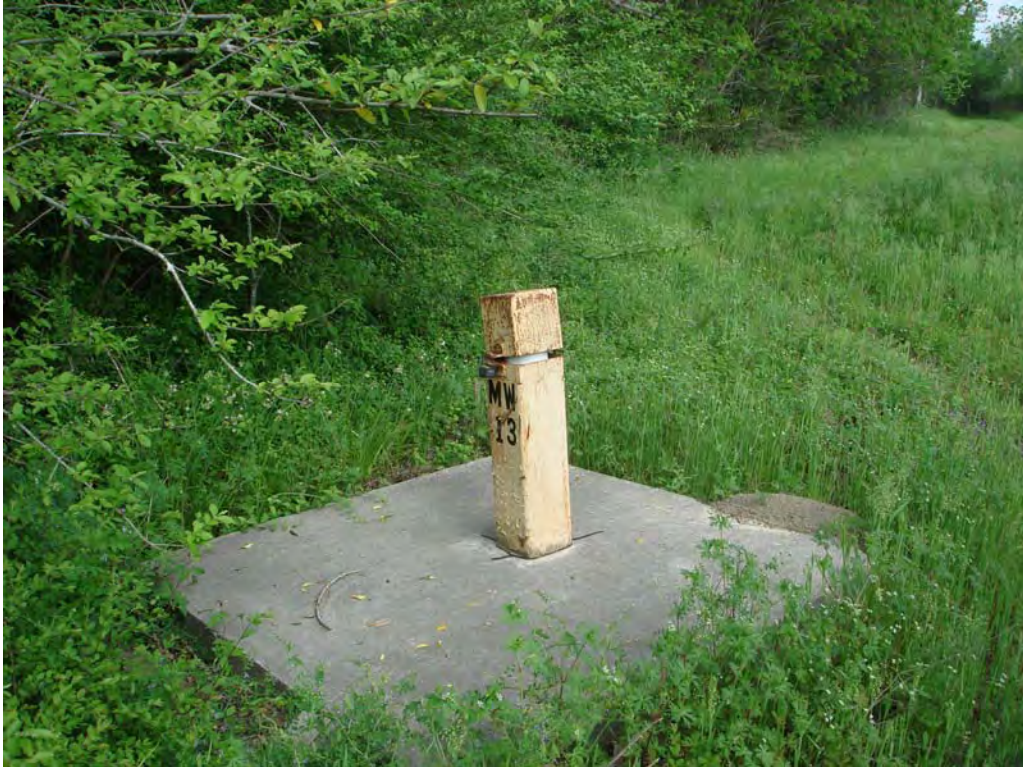
Photograph No. 7 Site: Dutchtown Treatment Plant Superfund Site Description: Monitoring well MW-13 north of site Date: March 29, 2007 (note gap caused by damaged hinge)
