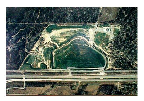
Scenic Site after cap is in place and seeded with grass. Eleven potential recovery wells have been drilled. Recovery pumps to be installed in some of these wells for collection of contaminated ground water in 1999, as part of future remedial actions to be implemented.
