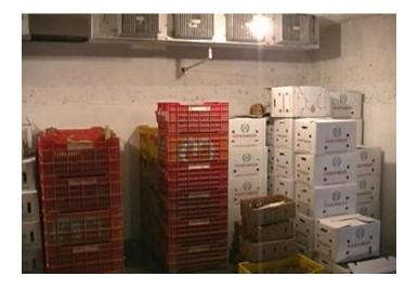
Room cooling is a slow and inefficient method of removing product field heat. A much faster and more effective cooling method is to use forced air. The rate of cooling may be up to 5 times faster using forced air versus room cooling. The cooling rate should be sufficiently quick to remove the product's field heat to near the optimal storage temperature within 1-2 hours after harvest.
