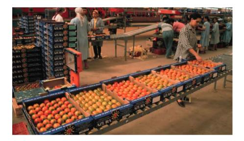
After packing and weighing the export cartons, they can either be moved individually on top of another roller conveyor to the cooling area, or put on a pallet which is moved by a hand jack to the cooler. Following cooling and/or temporary storage, the cartons can be moved by roller conveyor (or by hand jack, if palletized) from the refrigerated holding room and loaded directly into a refrigerated truck or marine container destined for the airport or seaport.
