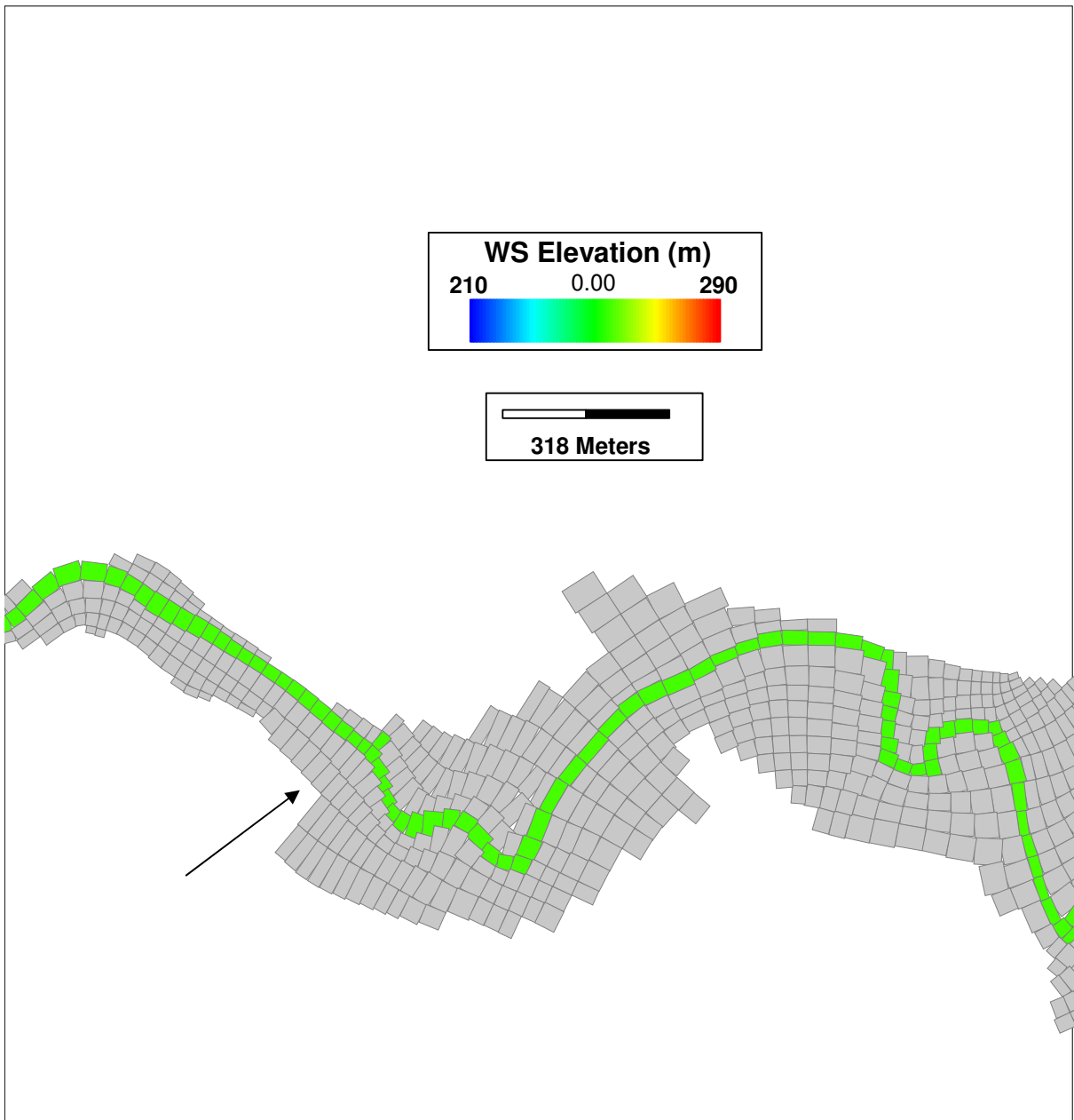
Figure C.6 Computation grid for EFDC model. The arrow points to the start of a much narrower floodplain downstream of the meanders. North is up in this figure.
