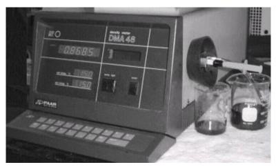
Figure 4 Digital densitometer taking a reading.
