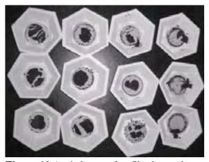
**Figure 10** Asphaltenes after filtering and drying.
