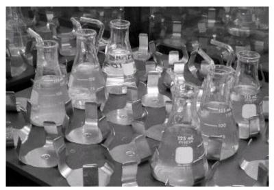
**Figure 8** Shaker flasks for dispersant effectiveness testing in shaker/incubator.
