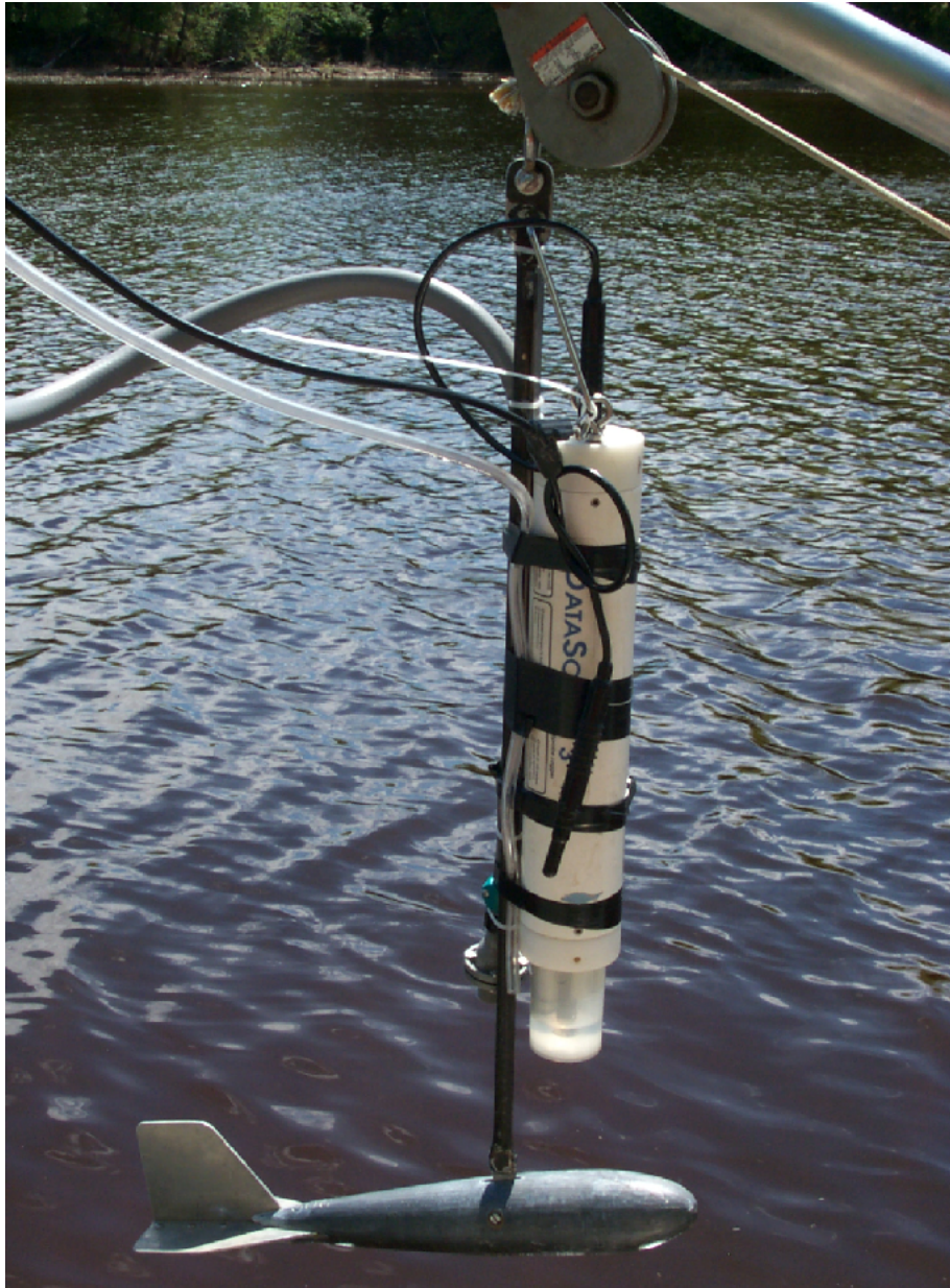
Figure 5-4. Apparatus for attaching instrument sensors and sample-collecting hoses to the sounding weight (30 lbs in this picture). A sounding-weight hanger-bar has been fabricated to accommodate a Hydrolab DataSonde. The DataSonde is attached to the hanger bar, facing forward, with stainless hose clamps (covered by tape in this picture). The hose to the peristaltic pump (small diameter) is taped to the DataSonde. The hose to the high volume Guzzler pump (large diameter) is attached to the hanger bar with plastic cable ties. A one-way valve is attached to the end of the Guzzler hose. When the apparatus is lowered, the instrument cables and hoses are attached to the winch line with cable ties. Other configurations are acceptable.
