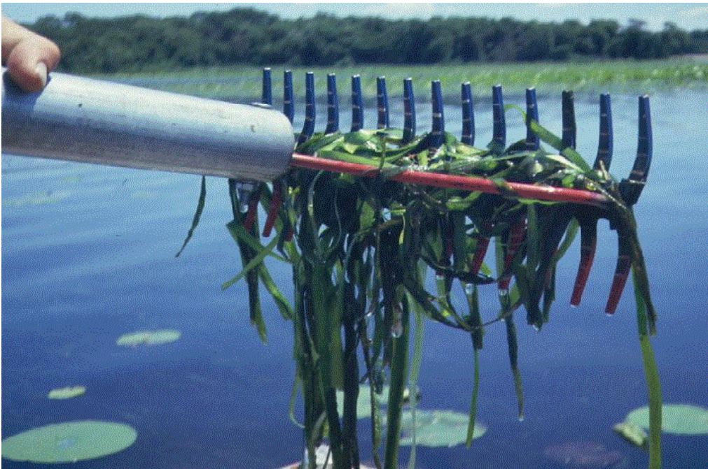
Figure 6-2. Double-headed sampling rake. Each tine is marked into 5 sections of equal length. In this sample, total density would be scored as "2" based on rake fullness.
