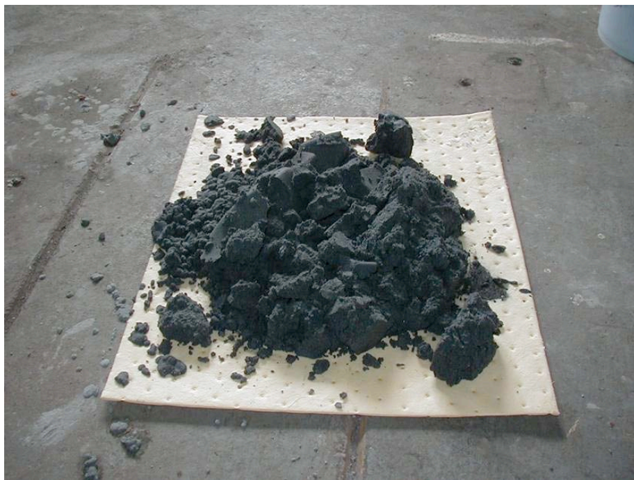
Photo 10 – Wet, treated sediment dewatered in filter press
