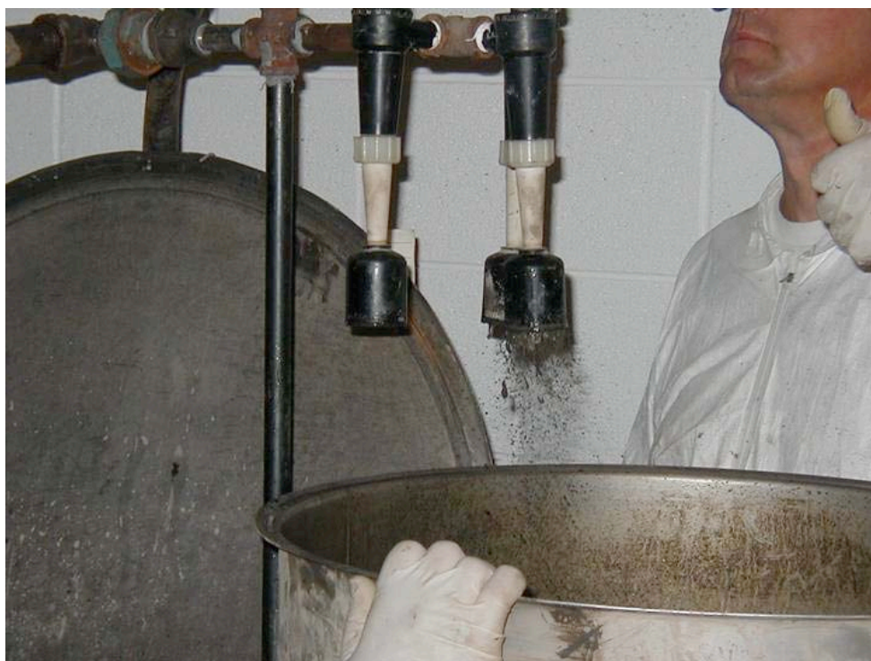
Photo 6 – Hydrocyclones over shaker screen
