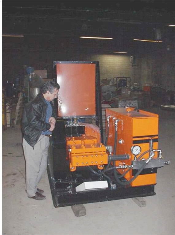
Photo 3 – Water blaster pump
